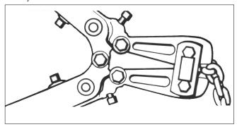
Figure 15. Cutting Chain with a bolt cutter
