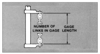
Figure 10. Gaging Load Chain Wear
