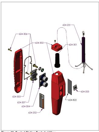
Figure 16. Control Station Exploded View
