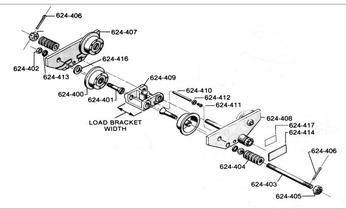
Figure 18. Series 635 Low Headroom Trolley Exploded View
