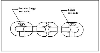
Use only CM Star (P) Grade Load Chain and CM replacement parts. Use of other chain and parts may be dangerous and voids factory warranty.
