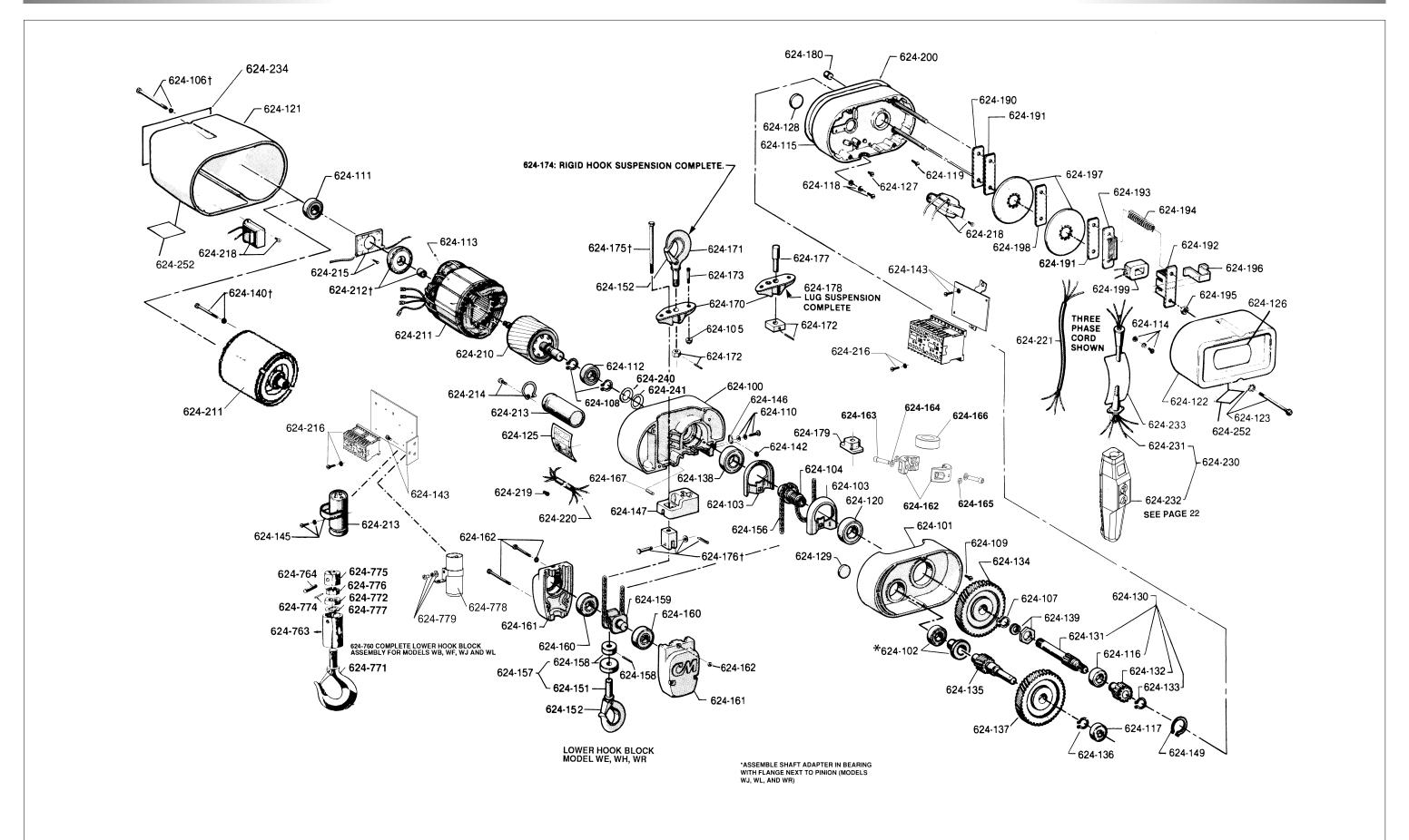
Figure 17. Valustar Electric Chain Hoist Exploded View
