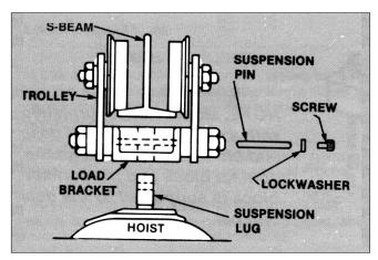
Figure 8. Attaching Hoist to Trolley
