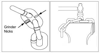
Figure 14. Cutting Chain by nicking
