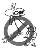
Be sure load is hooked securely Do not tip load the hook. Do not load hook latch. Hook latch is to prevent detachment of load under slack chain conditions only.
