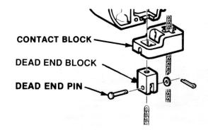
NOTE: Model WR is furnished with a contact block. The dead end block passes through the contact block and the contact block is supported by the dead end pin.
